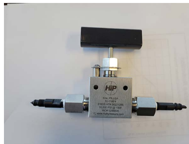
Outlet Valve Stem Assembly (#171-83-2)
